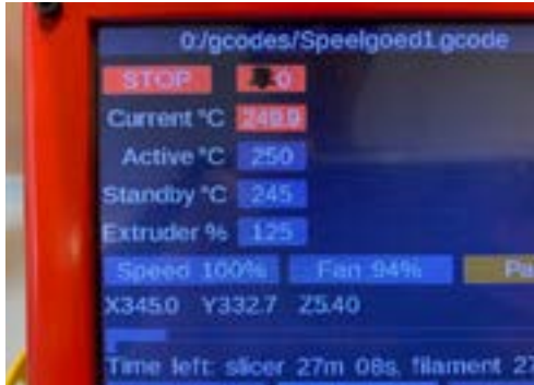
Picture 18: Example of printing settings using a recycled spool.
