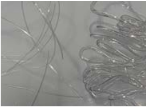
Picture 15: Same mixture of PET and PETG plastic: on the left using vacuum formed and on the right blow-molded
