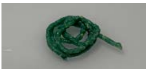
Picture 10: Low temperatures can push the material better out of the nozzle. However in this case 230 degrees was not enough to melt the plastic fully.
