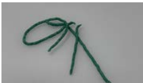
Picture 11: Test to see how low the temperature can be to be fully molten, the extra 5 degrees were still not enough.
