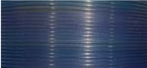
Picture 16: Mixture of 80% PETG and 20% colored PET gives a good result to produce filament, this further confirms that the higher concentration of vacuum-formed PET is what causes the disruption of the filament making process.
