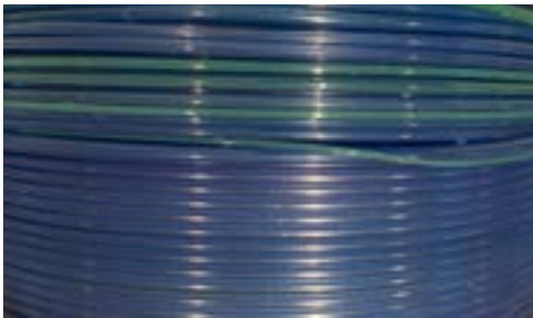
Picture 17: easily noticeable by the green color, the new mixture suddenly becomes thinner and thinner until it cannot be spooled anymore.
