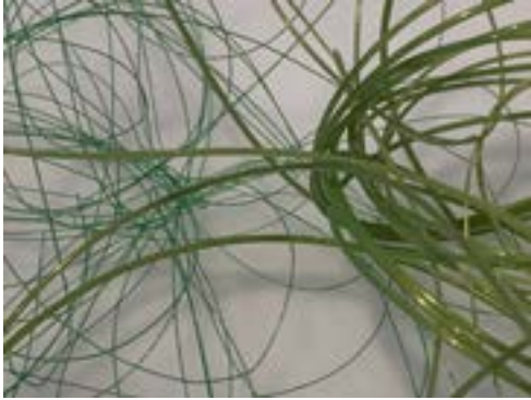
Picture 14: Same mixture of PET and PETG plastic but on the left using vacuum formed and on the right blow-molded
