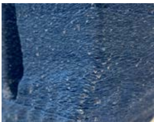
Picture 17: Printing with a spool that contained too much humidity, as well as contamination from other plastics, thus causing the white specks.
