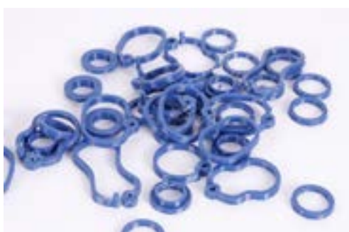
Picture 19: PET is flexible which allows us to print tie wraps.
