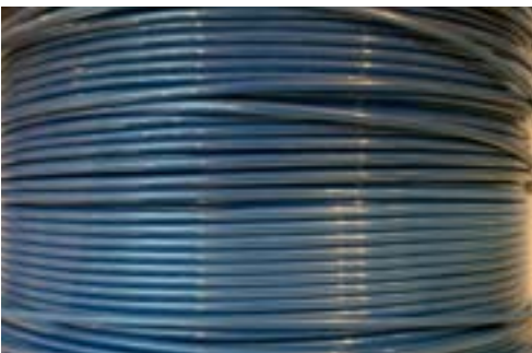
| Picture 13: Spooled filament with consistent diameter and perfectly aligned in contrast to the errors showed above.
