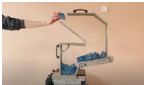
| Picture 3: Example of material accumulating in the shredder
